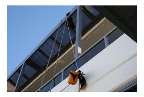
View of deviation anchor with rope protector clearly shown jammed in connecting carabiner. Note that backup rope has at some point during the incident, flicked behind the adjacent deviation anchor. There is no indication of the backup line or device being loaded during the incident
