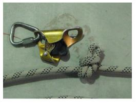
the operator in order to isolate out a damage point in the working rope. The exact position of this alpine butterfly relative to the second deviation (after the extra rope was added into the system by the rooftop operators) is unknown. The picture at right shows this knot and the extreme capsizing and cinching that has occurred. The Croll is orientated in the direction the alpine was orientated at the time of the fall i.e. left / up.
